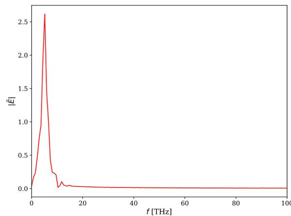
Figure 3: The Fourier transform of the electric field generated by the drive bunch.
