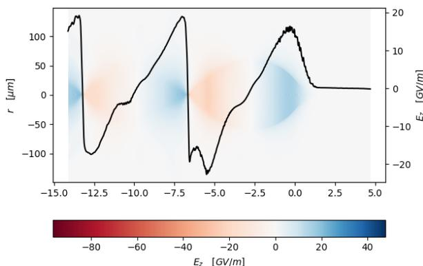
Figure 5: Blowout PWFA with a loaded wake.
