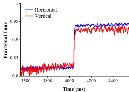
Figure 5: Calculated tune shifts at the all beam loss.
