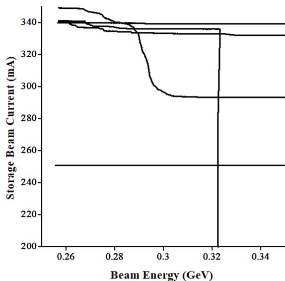
Figure 1: Beam loss at the energy ramp-up.
