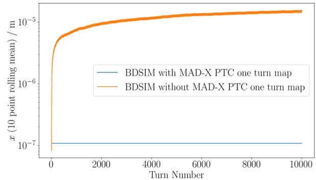
Figure 2: BDSIM long term tracking comparison for a reference particle. The transverse position  $x$  is recorded at the end of each turn for 10,000 turns with and without the use of a one turn map to correct the particle's trajectory.
