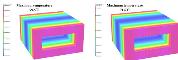
(a) laminated steel without slits (b) laminated steel with slits
