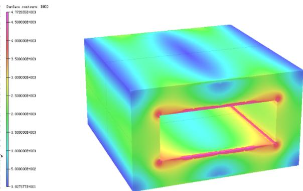
Figure 8: The field distribution of MnZn ferrite.
