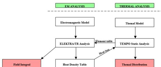
Figure 2: Procedure of electromagnetic and thermal analysis.
