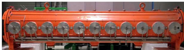
Figure 2: 11-cell section of the accelerating TWS.
