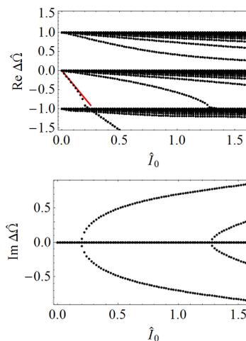
Figure 1: Classical TMCI in the absence of HHCs: real (top) and imaginary (bottom) parts of the mode complex-number frequency shift  $\Delta\Omega = (\Omega - \omega_y)/\omega_{s0}$  over a bunch-current range. The red line in the top picture is the tunes shift for the rigid dipole mode as given by Eq. (7).
