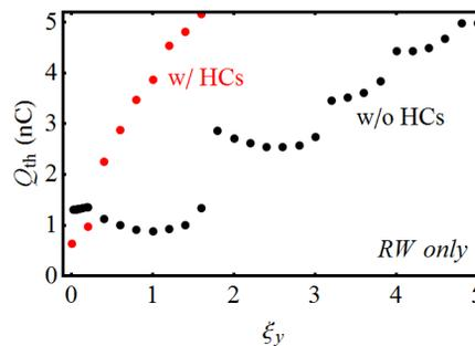
Figure 5: Single-bunch instability threshold vs. chromaticity with and without HHCs (ALS-U studies). *Elegant* [12] simulation. The presence of HHCs considerably enhances the stabilizing effect of a finite positive chromaticity. Radiation damping included.
