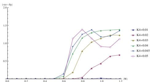
Figure 2: Showing the magnitude of net spin loss after accelerating through the primary resonance. This is plotted against the spin resonance magnitude of the primary resonance  $|w|$  (proportional to the action or emittance of the particles). We see the effect of changing the neighboring resonance.
