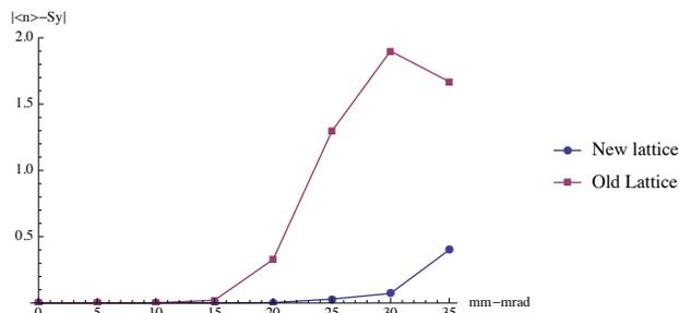
Figure 3: Polarization deviation from invariant spin field direction versus emittance curve after crossing  $G\gamma = 422.685$  spin resonance. Comparing old RHIC 255 GeV lattice (old lattice) to optimized lattice (new lattice).
