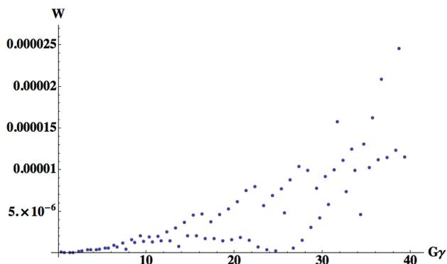
Figure 4: Plot of intrinsic spin resonances versus  $G\gamma$  for a particle of 10 mm-mrad normalized emittance. This is the result of spin optimization code SOptim applied to the RCS lattice after applying symmetry breaking detector bypasses.
