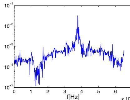
Figure 8: Sidebands in the vertical tune spectra for  $\rho_e = 5 \cdot 10^{12} \text{ N}_e/\text{m}^3$ .
