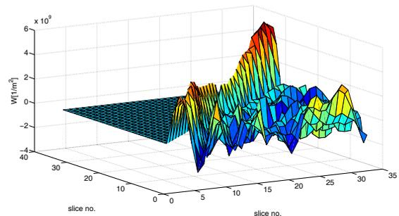
Figure 3: Wake matrix for  $\rho_e = 5 \cdot 10^{12} \text{ N}_e/\text{m}^3$ .
