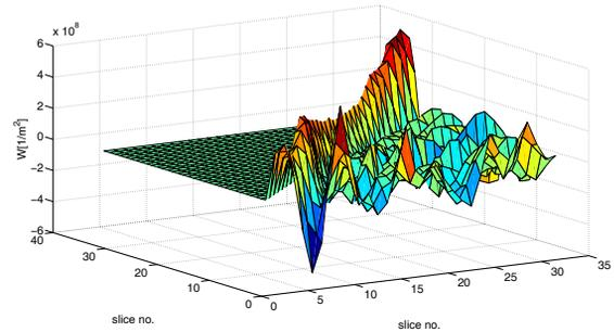
Figure 2: Wake matrix for  $\rho_e = 5 \cdot 10^{11} \text{ N}_e/\text{m}^3$ .
