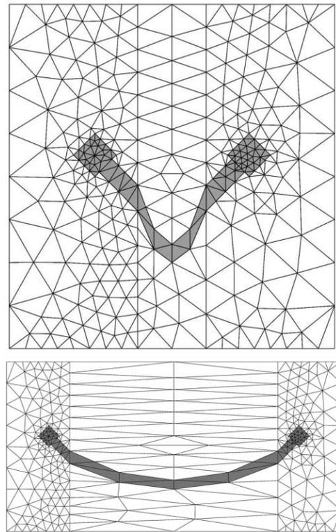
Figure 7: Example of one and the same finite element mesh generated for in the domain of two different charts. The upper domain appears shorter than the lower one implying mesh generation is easier in the upper one.
