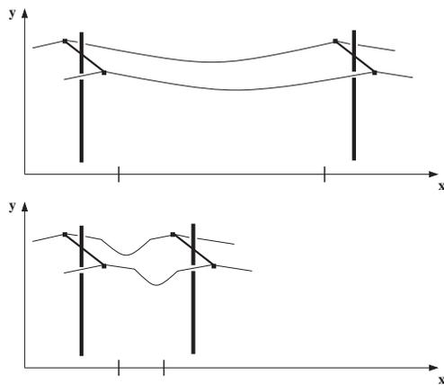
Figure 6: One and the same electric power line (point set) represented in different coordinate systems. The difference lies in the metric of  $\mathbb{R}^n$  which is not chosen the same way in the region between the poles –i.e., in the area between the ticks on the  $x$ -axis. Still, both charts map to one and the same point set. Consequently, both charts can be employed to solve the electromagnetic fields generated by the power line. However, generating the mesh is easier in the lower domain.
