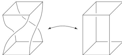
Figure 5: To compute fields caused by twisted objects, all one needs is to give meaning to the constitutive law by introducing a transition map between a straight bar and the twisted object.
