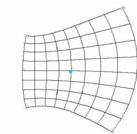
Figure 9: The same field but the shape of the plates has changed. This new shape is found by solving for Euclidean coordinates without changing the electric chart.
