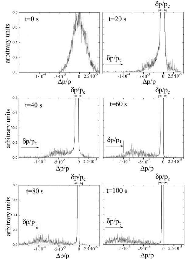
Fig.1. The evolution of the momentum distribution in the HESR at energy of 8 GeV. The effective pellet target thickness is  $5 \cdot 10^{15}$  cm<sup>-2</sup>. The electron cooling and IBS are switched on.
