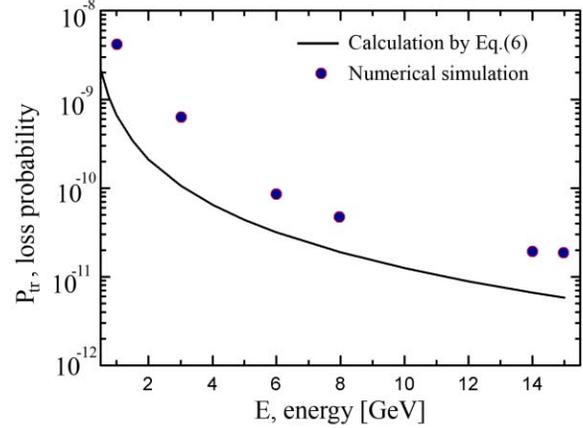
Fig.6. The probability of transverse beam loss per turn assuming the ring acceptance of 10 mm mrad.
