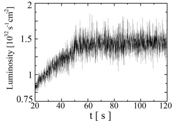
Fig. 3. The luminosity versus time calculated every 20000 turns. The effective target density  $n_t = 5 \cdot 10^{15} \text{ cm}^{-2}$ ,  $N_i = 10^{11}$ ,  $E_{\text{kin}} = 8 \text{ GeV}$ .
