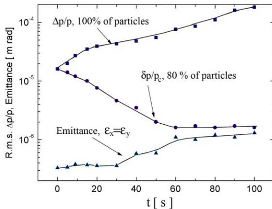
Fig.2. The time evolution of the momentum spread and emittances of the beam at energy of 8 GeV in the HESR including electron cooling and IBS.
