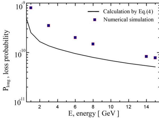
Fig.5. The probability of longitudinal beam loss per turn assuming  $\Delta p/p_{acc} = \pm 5 \cdot 10^{-4}$ .
