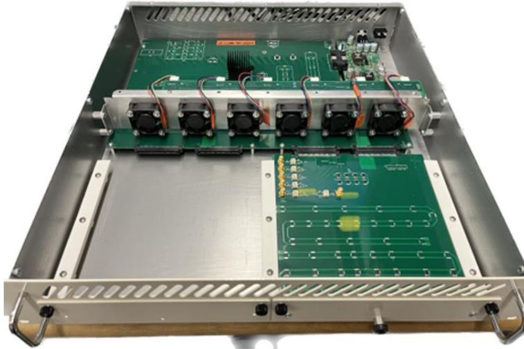
Thermal/Airflow Mockup Chassis
