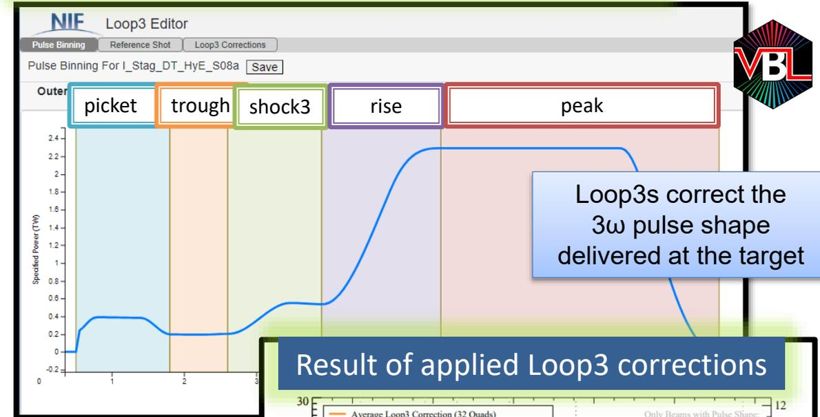
In this example, power accuracy was improved by adjusting the request in the picket, trough, and shock3 regions of the pulse, using data from a prior shot in the same campaign
