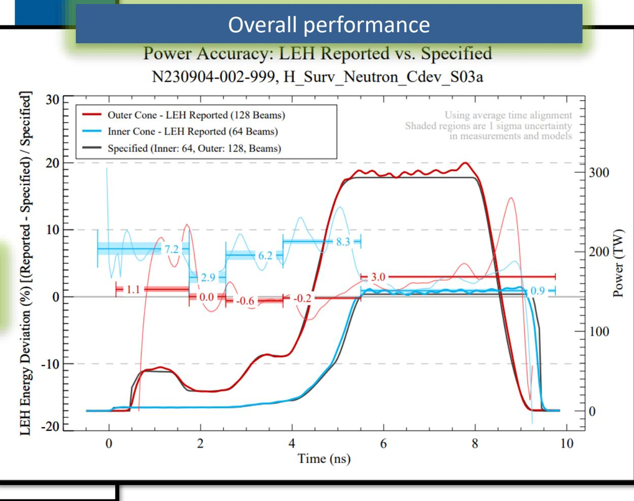
The accuracy and timing of the delivered pulses onto the target directly affect the symmetry of the implosion critical to achieve fusion ignition
