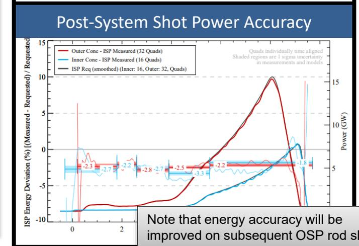
Automated loop1 corrections improve performance without requiring time consuming manual work by the laser physicists
