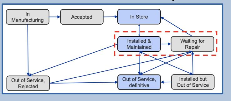
A failure is deemed to have occurred when and Maintained" to "Waiting for Repair", as shown in the EAM state machine above.
