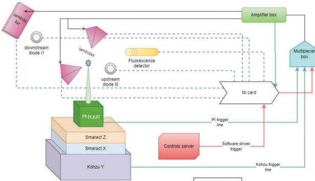
Software and signals scheme for the experiment setup on P07, PETRA III
