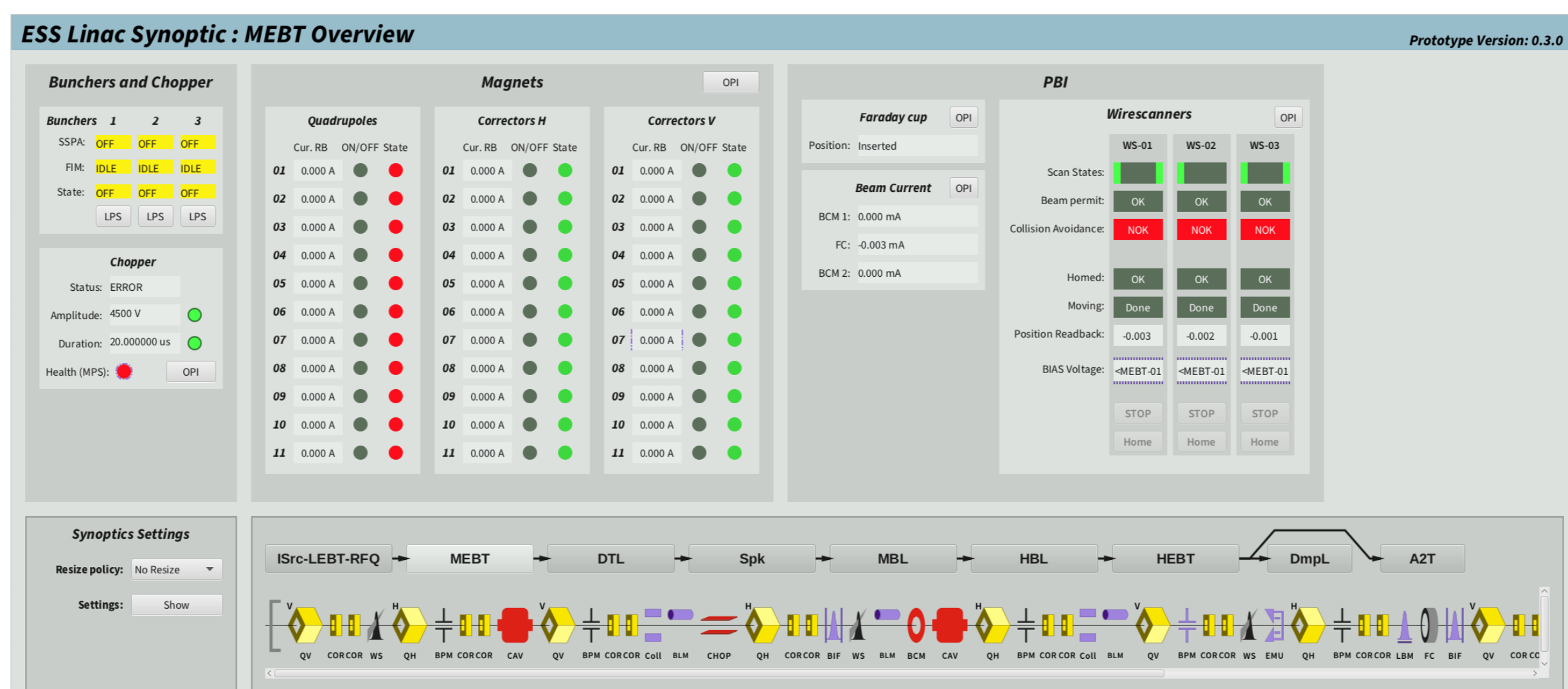
Fig. 4. The Accelerator Synoptics Interface showing the high-level overview of the Linac MEBT section.
