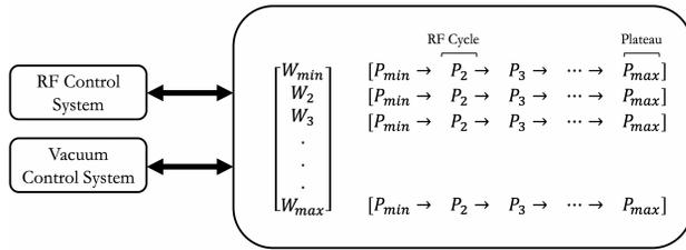
Figure 5: Conditioning application width ( $\vec{w}$ ) and power vectors ( $\vec{P}$ ).
