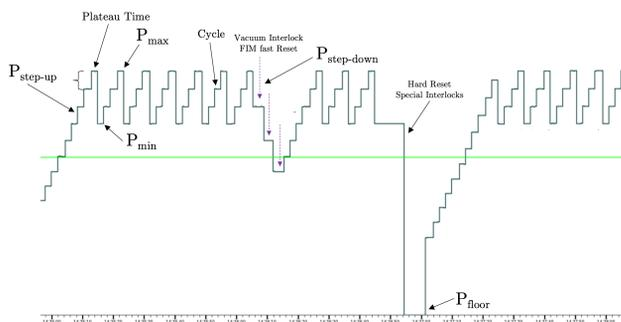
Figure 7: Example from DTL conditioning showing the different algorithm parameters, ramp-up, ramp-down and hard-reset procedures.
