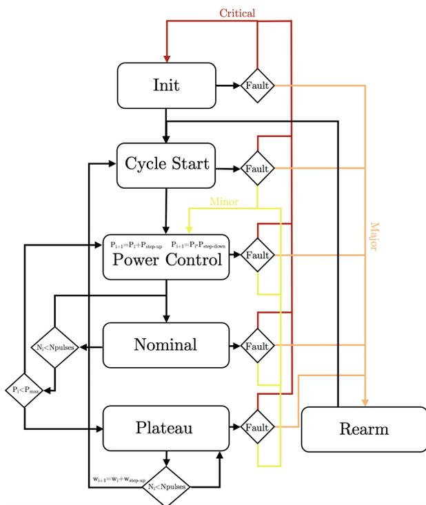
Figure 9: RF conditioning algorithm flowchart.
