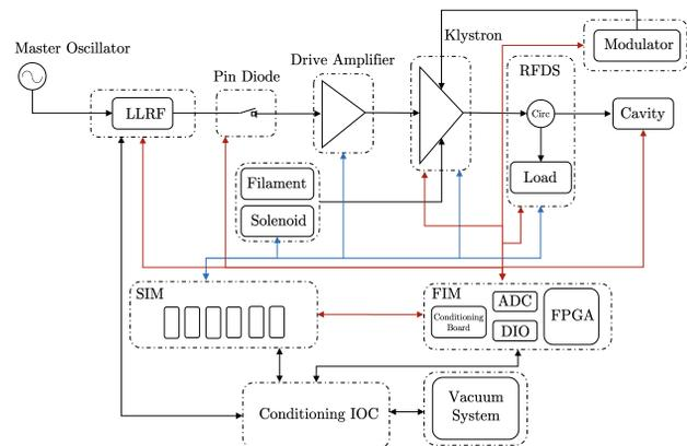
Figure 4: RF cavity simplified control system architecture.
