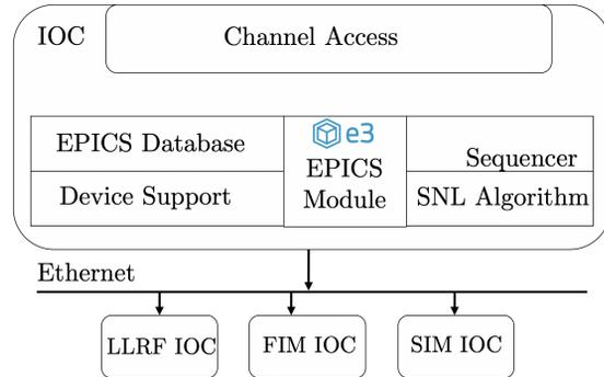
Figure 3: Conditioning algorithm IOC structure.
