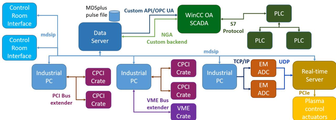
Figure 2: The new CODAS architecture of RFX-mod 2.
