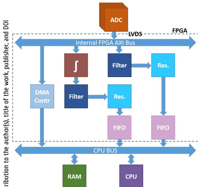
Figure 1: The FPGA architecture. DMA Controllers and FIFOs are implemented by XILINX IPs AXI-DMA and AXI4-FIFO, respectively.
