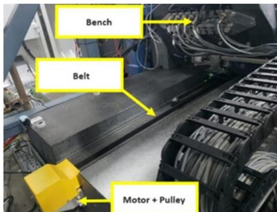
Figure 2: General assembly: bench, belt, motor and pulley.
