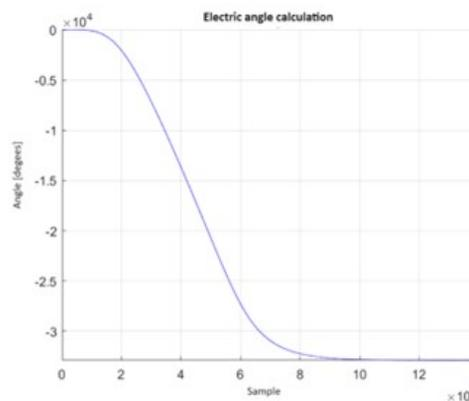
Figure 5: Electric angle calculation, from currents acquired.
