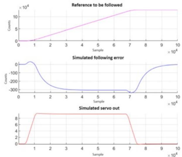
Figure 7: Expected results after controller design. Simulation done using Simulink.
