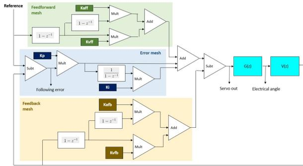
Figure 6: Controller standard structure inside PBLV to be simulated in Simulink.
