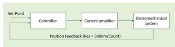
Figure 3: Resumed block diagram of the system.
