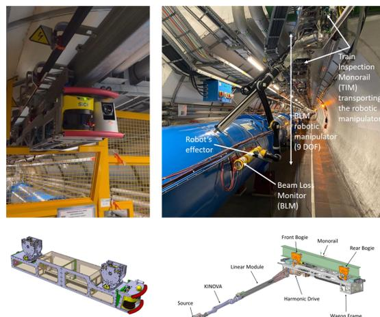
Figure 6: TIM robot passing the LHC sector doors (top left), 3D view of a TIM wagon (bottom left), 9 degrees of freedom robotic wagon (top right), 3D view of the robotic wagon (bottom right).
