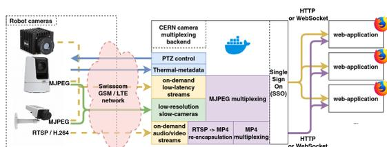
Figure 5: Novel framework developed for camera images streaming from the TIM robot.
