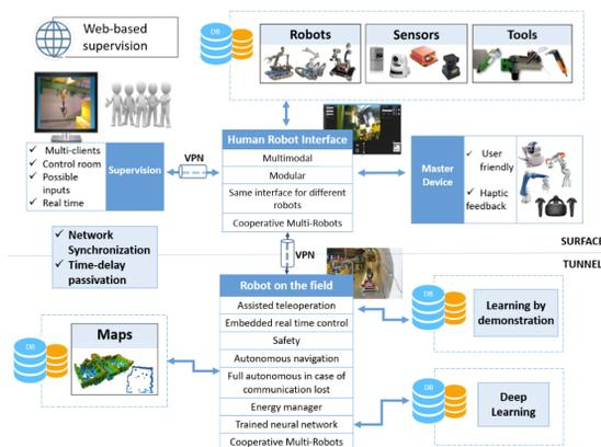
Figure 2: CERNTAURO framework architecture. The robot has an onboard intelligent control featuring capabilities like autonomous navigation and energy management.
