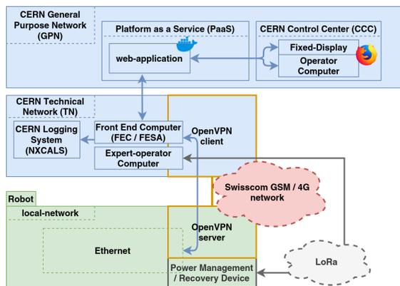
Figure 4: Control scheme for the robots integrated in accelerator controls infrastructure.
