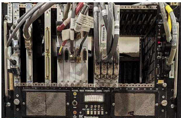
Figure 3: CAMAC Crate to be replaced by Moxa ioThinX.
