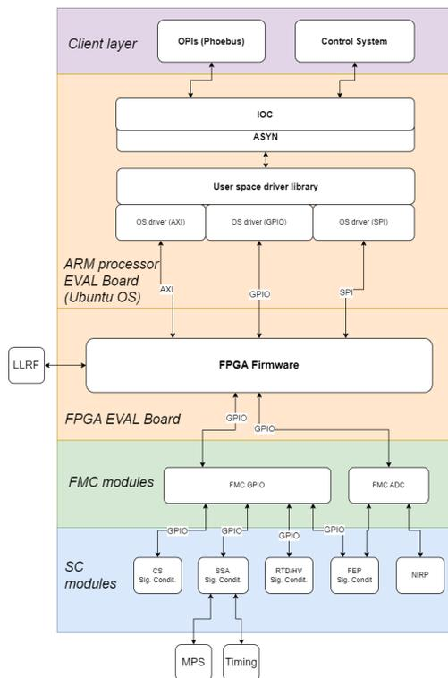
Figure 8: The main logic unit software diagram.
