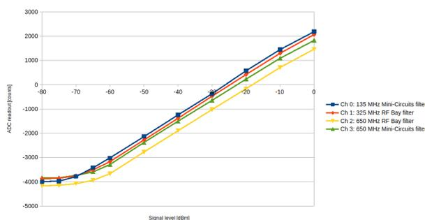
Figure 7: The RF detector characterization for different pass-band filters used in the design.
