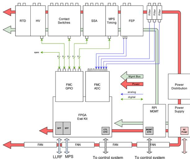
Figure 1: The block diagram of the PoC structure.
