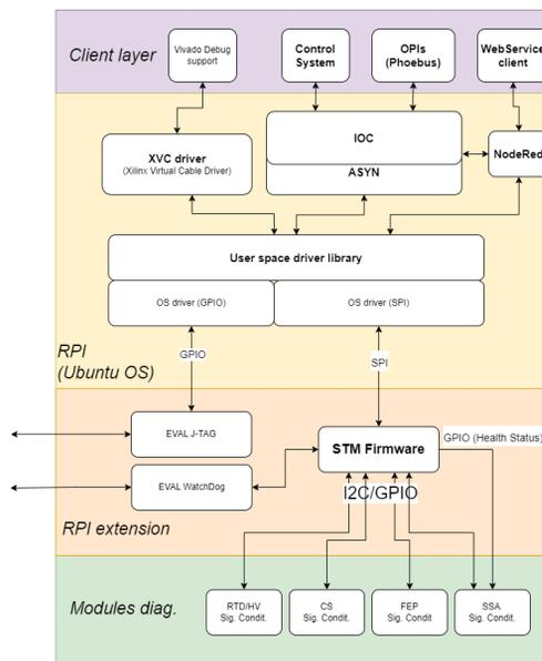
Figure 9: The management and diagnostics SW diagram.
