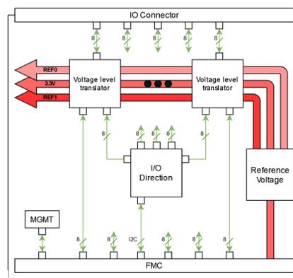
Figure 2: The FMC GPIO module block diagram.
