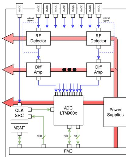
Figure 3: The FMC ADC module block diagram.
