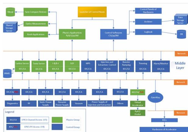
Figure 1: The control system architecture diagram of HEPS.
