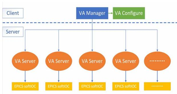
Figure 2: The framework of Multi-User Virtual Accelerator.
