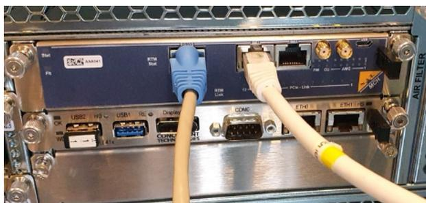
Figure 3: Picture of 3U chassis with MCH connected.
