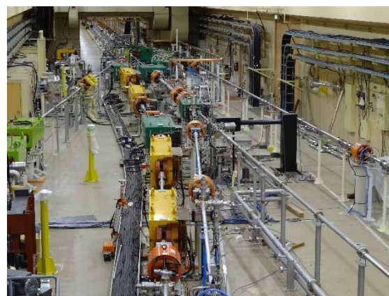
Figure 2: Photograph of the third beam switching yard at the KEK e-/e+ injector LINAC. The LINAC beam line branches to the beam transport lines with the deflecting pulsed bending magnet.
