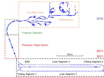
Accelerator Segments, staged commissioning: 2017 ECR ion source 2017 Front-End (FE), 0.5 MeV/u 2018-2019 Linac Segment 1 (LS1), 20 MeV/u 2020 Folding Segment 1 (FS1) 2020 Linac Segment 2 (LS2), 200 MeV/u 2021 Folding Segment 2 (FS2) 2021 Linac Segment 3 (LS3), > 200 MeV/u 2021 Beam Delivery System (BDS) 2021-2022 Target Systems, rare isotope beams! 2021-2022 Fragment Separator (ARIS)
