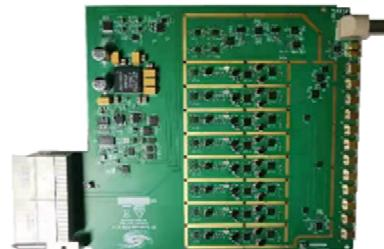
down-conversion and up-conversion RTM module.
