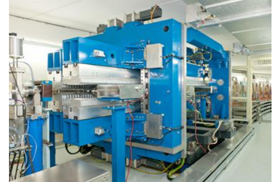
DEPU in SSRF
