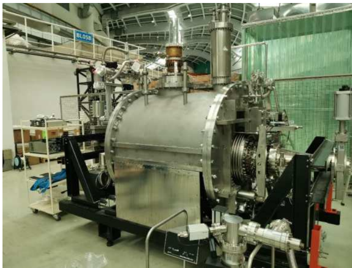
Fig. The 500 MHz SC cryomodule integration in the test tunnel
