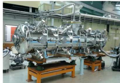
4m superconducting V-polarization undulator for SHINE
