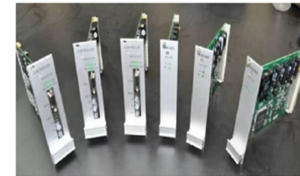
PS controller for SSRF and SHINE
