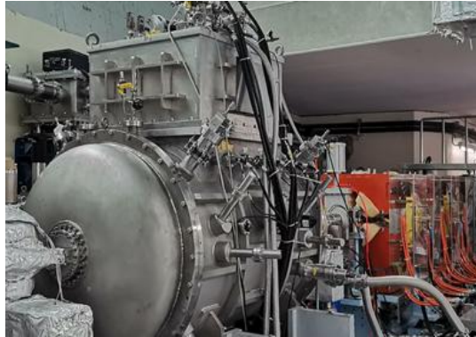
Superconducting undulator for SSRF
