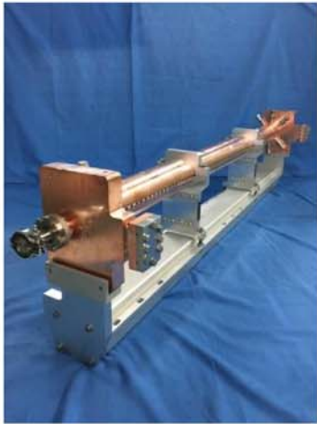
C-band high gradient accelerating structure for SXFEL 37MV/m on average, 41.7MV/m on maximum
