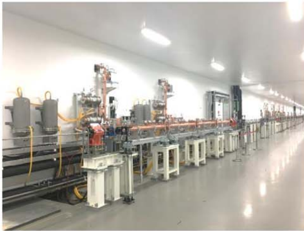
C-band high gradient accelerating structure for SXFEL 37MV/m on average, 41.7MV/m on maximum
