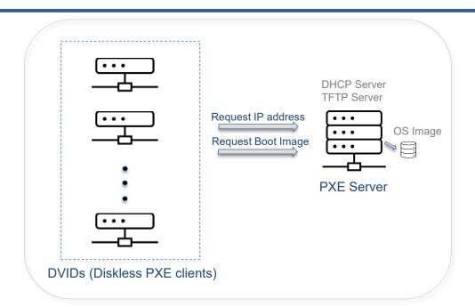
The diskless DVIDs network boot from a single Linux OS image solving the multiple image and HDD maintenance problem.
