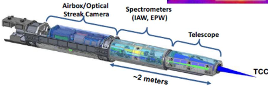
Optical Thompson Scattering (OTS): new instrument controls and automatic alignment for deep-UV (210nm) laser “plasma probe”: 400 devices, 3 new device types, 20 alignment loops
