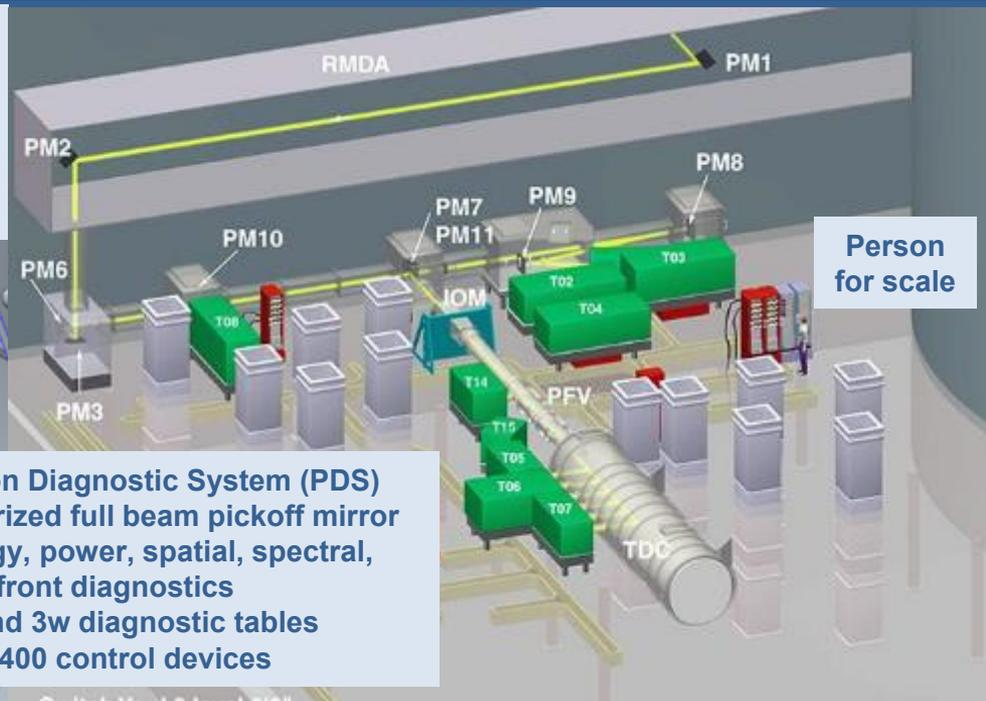
New instruments allow to measure with improved accuracy parameters of 3w ultraviolet light delivered onto the target, tune-up the laser and update calibrations for better energy balance
