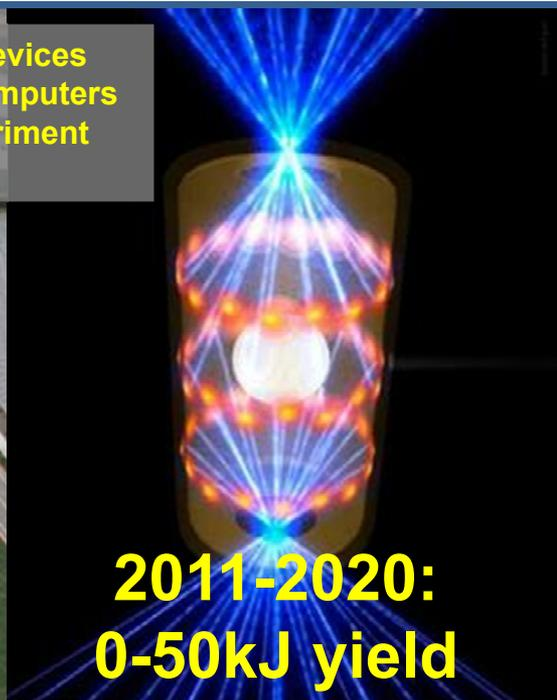
NIF, the world's largest and most energetic laser, is pursuing the goal of Ignition, when DT target produces more energy from fusion than laser drive input
