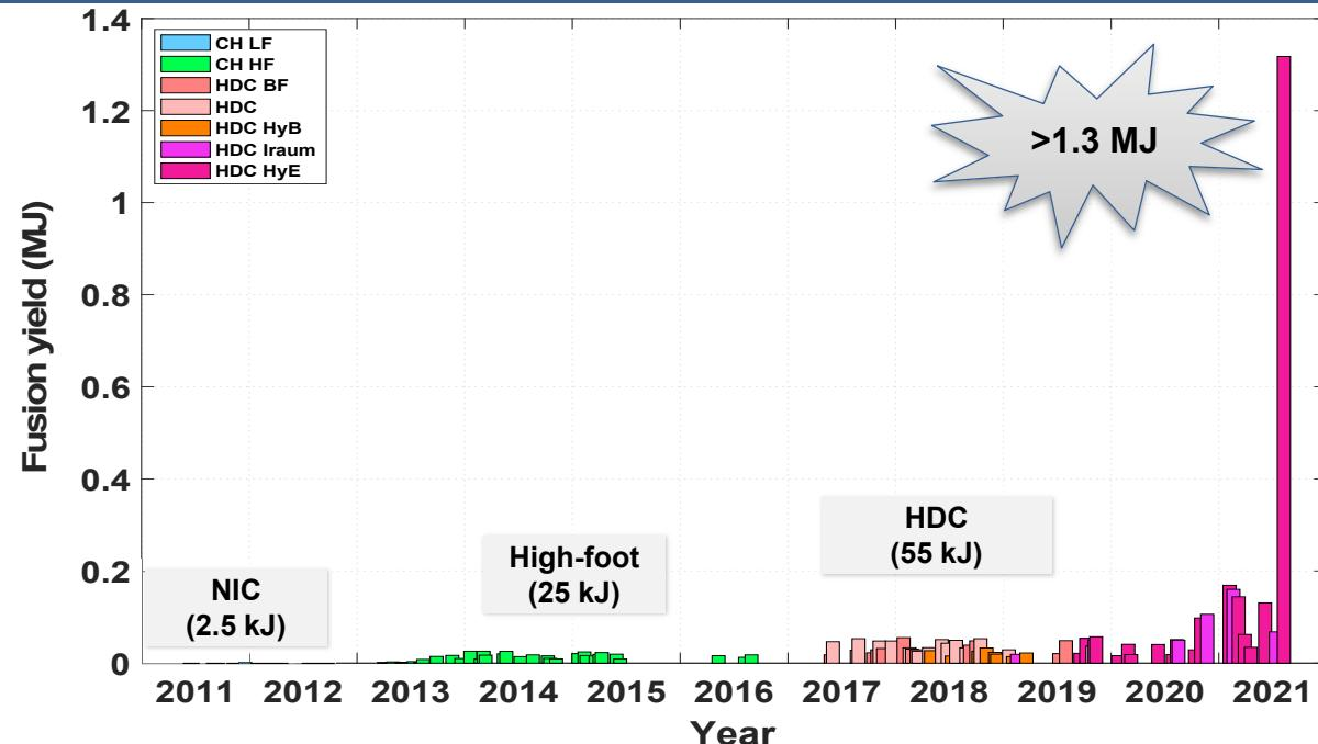
This latest experiment culminates a series of record-setting shots of 2020-21, breaking both the 100 kJ and 1 MJ barriers within a year
