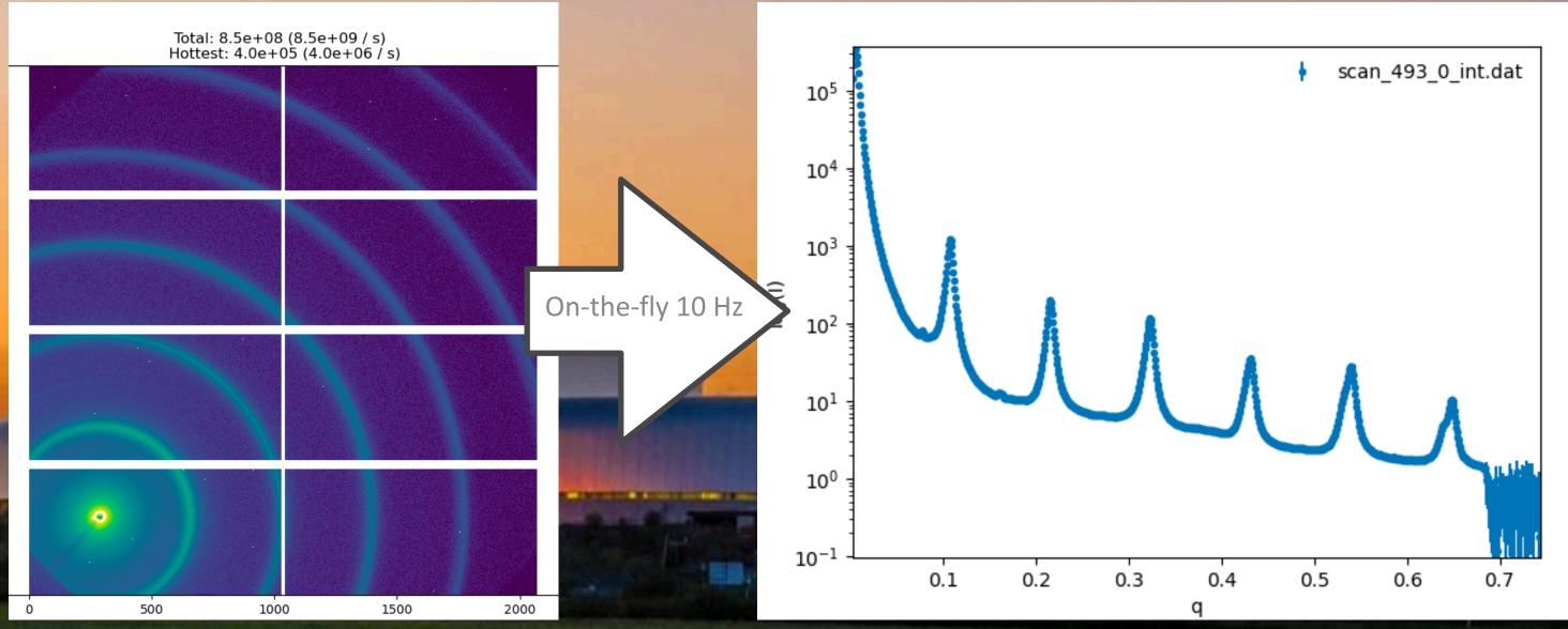
CoSAXS, Silver behenate use to calibrate SAXS data at short sample-to-detector distance. The Azimuthal Integration (right) shown in linear plot is computed on the fly at 10 Hz. (A. Terry)
