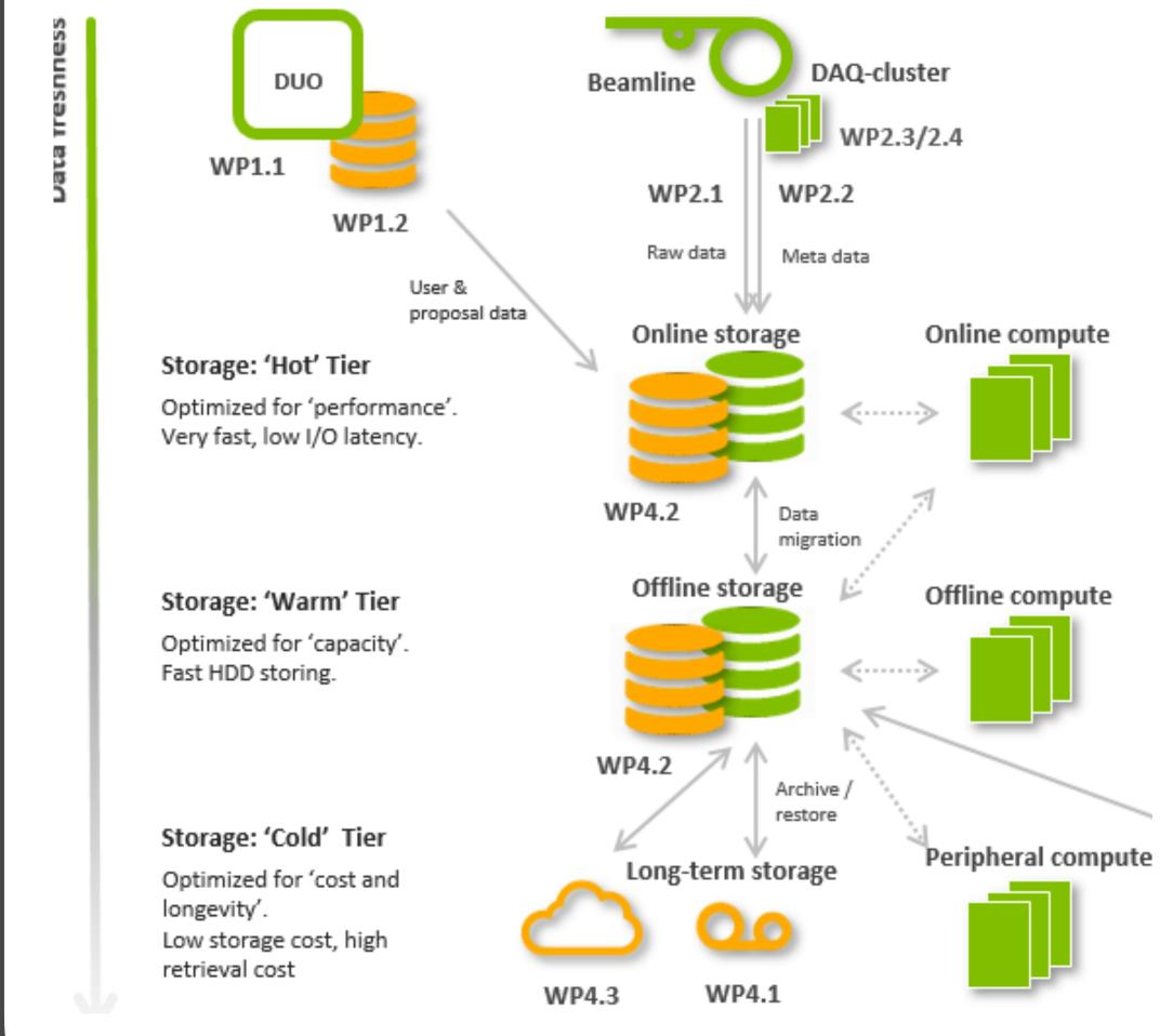
Main Upgrade of the Data Infrastructure: Performance and 10 years retention SciCAT is currently deployed on 9 beamlines
