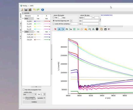
Balder, Copper foil EXAFS, Fly scan with a total accumulation time down to ~30 sec per full EXAFS. Parallel Execution of Sequential Data Analysis (right) is done online.
