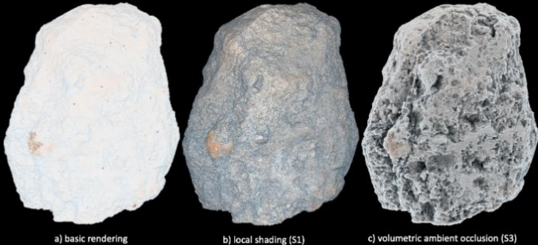
Figure 2: Soil sample renditions using Index XAC operators. (a) The original volume with basic rendering and no shading.(b) The volume rendered with XAC local shading (S1). (c) The more advanced XAC shading scheme with ambient occlusion(S3). Data courtesy: MOGNO beamline/Sirius, LNLS/CNPEM.
