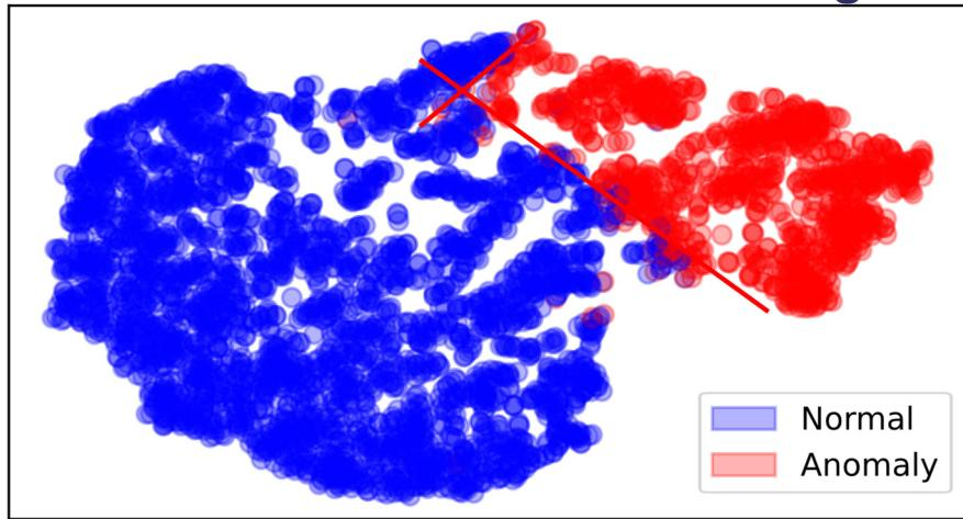
The generated class labels for each data point. Two approximate lines were used as a first pass for the class boundaries, and then a manual labelling process along the boundaries was used to make corrections.
