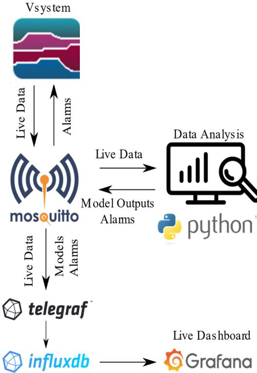
Software stack to apply to models and visualise the live data + model outputs in real time for operators.
