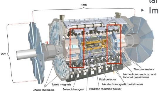
The New Small Wheel (NSW) upgrade will replace the current Small Wheel of the ATLAS muon spectrometer to handle larger particle rates
