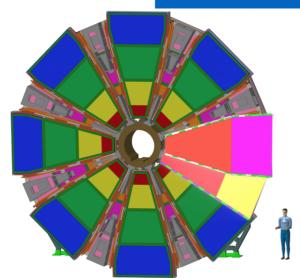
The NSW will provide high precision muon track reconstruction and trigger information to ATLAS, at high rates, thus eliminating the issues of the present SW.
