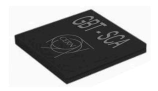
The GBT-SCA ASIC (Giga-Bit Transceiver - Slow Control Adapter) is the part of the GBT chipset which purpose is to distribute control and monitoring signals to the front-end electronics embedded in the detectors.
