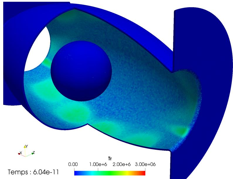
3D configuration simulation movie (D2 capsule and cavity)
