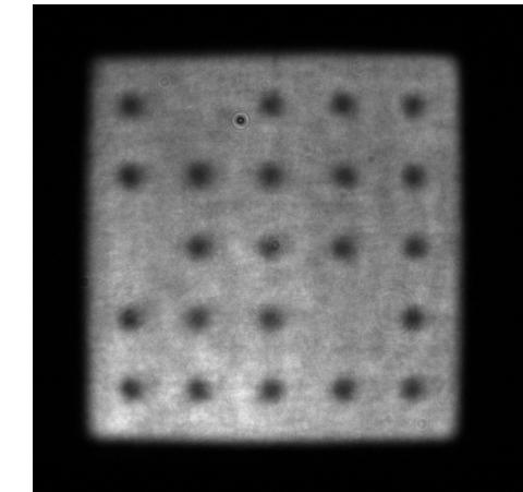
Spot blockers are being implemented to offer « manual » blocking capabilities on LMJ in 2020
