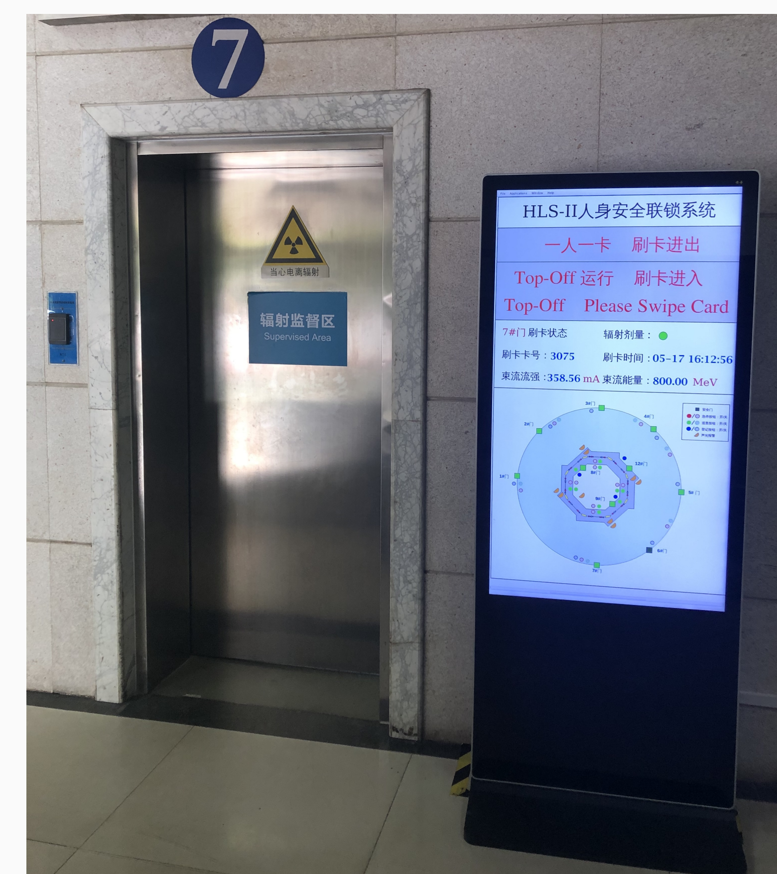
Fig. 5: Photo of the novel HLS-II PSS Door Display OPI
