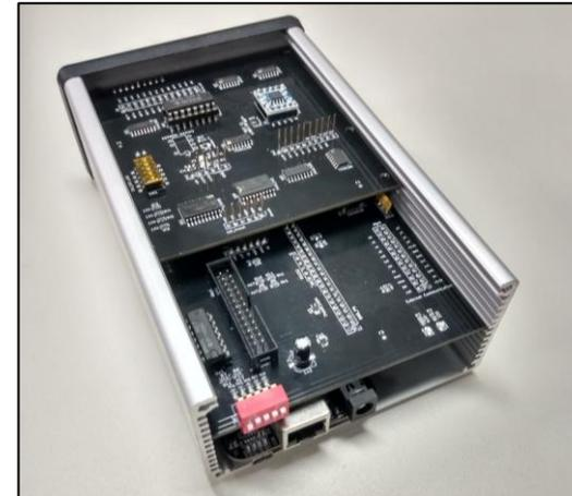
Figure 02: Assembled SIMAR unit (minus frontal panel) with interface and base boards
