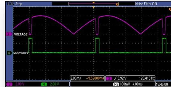
Figure 12: Voltage glitch detector using a derivative circuit.
