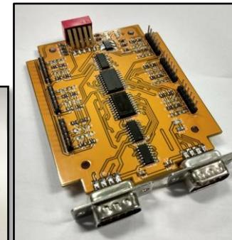
Figure 06: SPI/Serial expansion board
