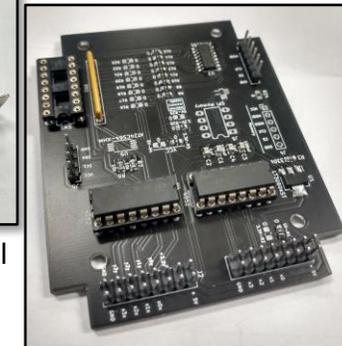
Figure 07: I<sup>2</sup>C Expansion Board
