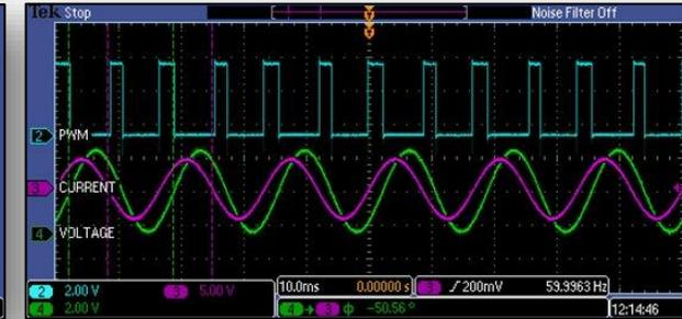
Figure 13: Power factor measurement based on a PWM circuit.
