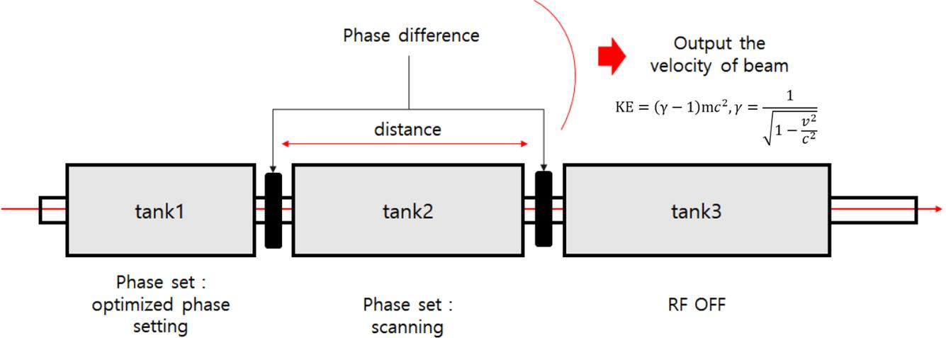
The beam energy from the measured RF phase
