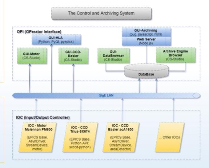
The control of the Beam Profile Station for Gamma Beam diagnostics includes one Mclennan PM600 motor controller and two Trius-SX674 CCD cameras.
