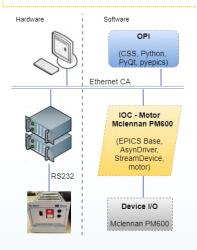
Mclennan PM600 is supported by the EPICS device support module motor record. The IOC can:
