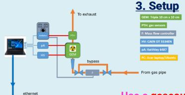
**Knowing the exact relation** between effective gas gain and gas concentration, it is possible to get the Ar/CO2 ratio of the supplied gas!
