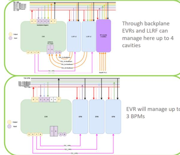
Through backplane EVRs and LLRF can manage here up to 4 cavities
