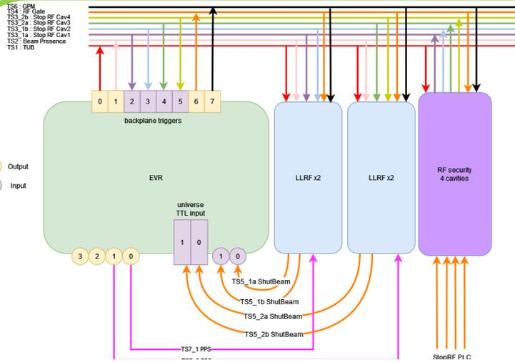
Through backplane EVRs and LLRF can manage here up to 4 cavities
