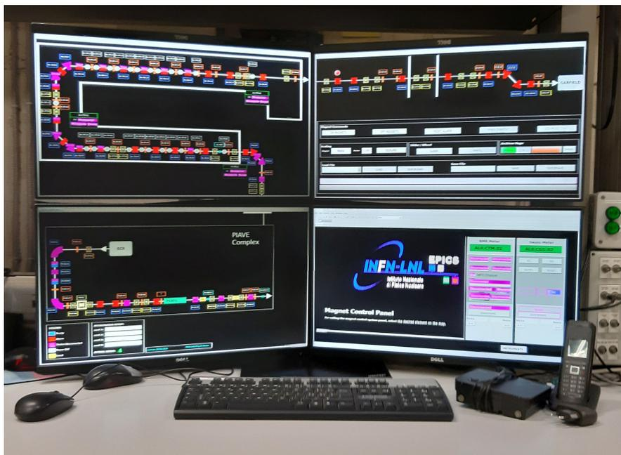
Many of these interactions are repetitive ( ex.: correct a current, change slits position, change RF parameters and move into another page of the GUI ) and they are commonly performed by mouse and keyboards connected to a common personal computer. Sometimes these tools are not the best solution for the operator: the biggest problem observed is the eye-hand coordination between mouse/keyboard and the multi-screen monitor
