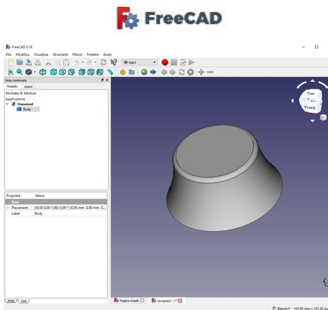
The KNOB 3D model designed in FreeCAD.
