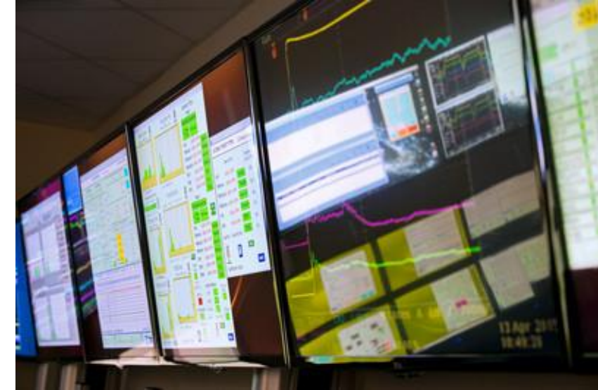
Figure 3: Example Vsystem screens in the ISIS main control room where alarm status of channels / PVs will be displayed
