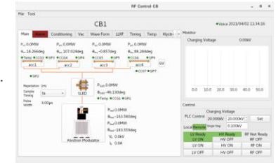
Figure 5: RF control GUI for C-band
