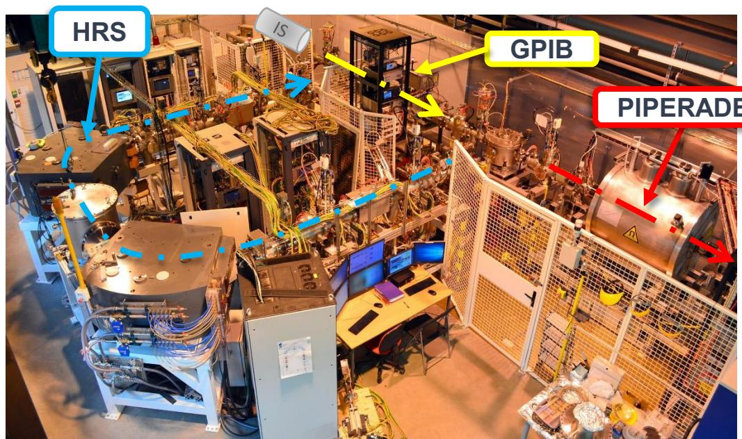
3 main devices are currently developed to guaranty high purity beams
