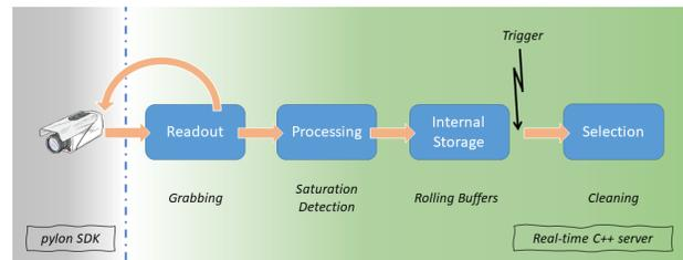
Figure 3: Image acquisition software model.
