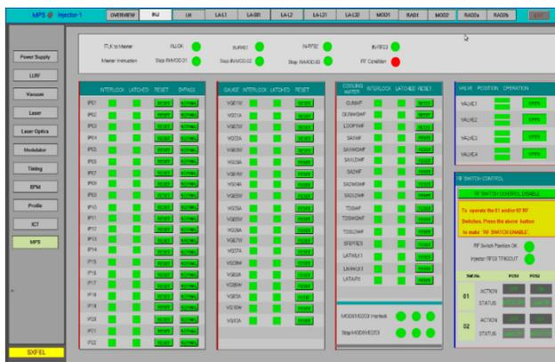
Figure 6: The interface of interlock system for SXFEL injector.
