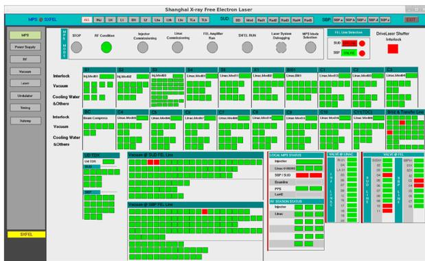
Figure 5: The global interface of SXFEL-UF MPS.
