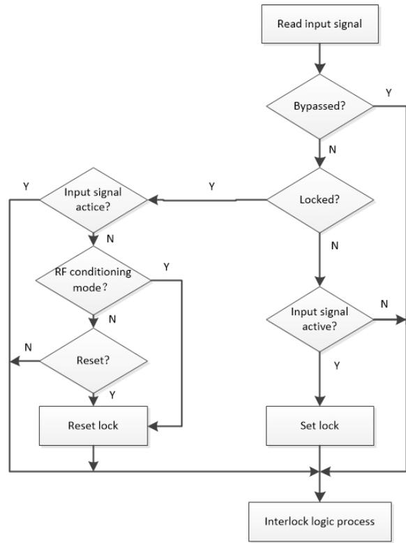
Figure 4: Flow chart of input signal process.
