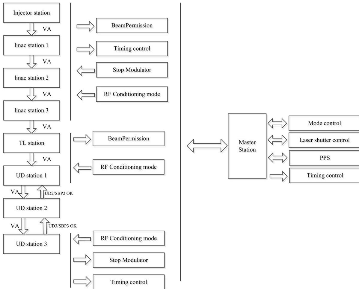
Figure 2: The structure of stations and signal interaction.
