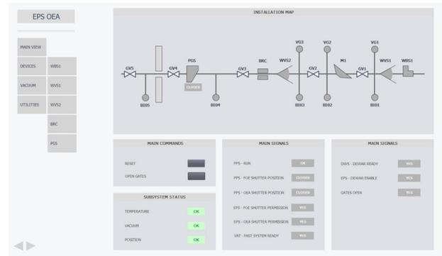
Figure 4: The main screen of EPS HMI of a hutch from a beamline representing a P&ID simplified diagram with components status, protection logics status, reset button, and the main interface signals between EPS and PPS.
