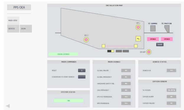
Figure 5: The main screen of PPS HMI showing FE's shutter status and components status inside the hutch, main diagnostic internal signals, interface signals with EPS, reset button, oxygen, and search status.
