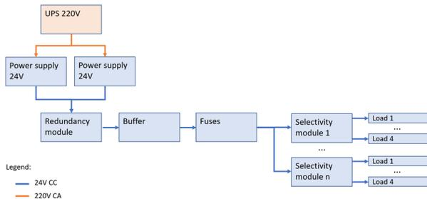
Figure 1: EPS and PPS's 24 VDC connection diagram.
