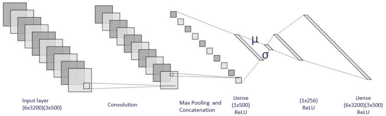
Figure 3: For the CERN XBOX data, three of the input channels were of a lower dimension, and each channel was processed by a CNN with filters of size  $1 \times 5$ , with the resulting feature vectors flattened and concatenated before being passed to a dense ReLU layer and encoded into the latent space. The decoder is constructed of a single dense ReLU layer with each channel consisting of a linear dense layer.
