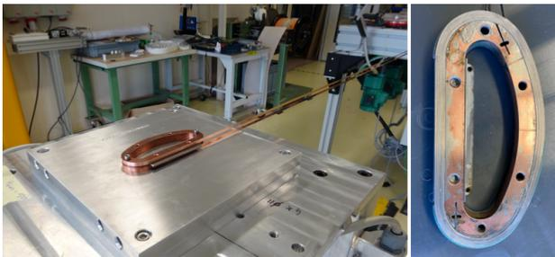
Figure 7: a) Winding of the first VR coil, b) The final coil after the soldering process.
