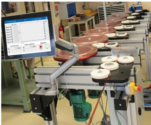
Figure 4: Winding machine with touch-panel user HMI.
