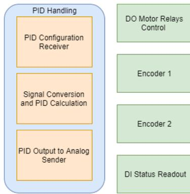
Figure 3: FPGA application parallel processes.
