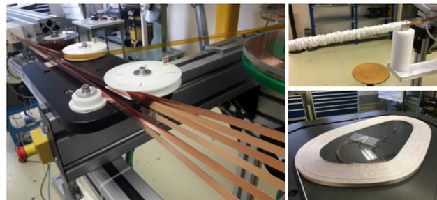
Figure 9: a) The winding machine with the 6 tapes, b) The S-2 Fiberglass stored on the tapes path, c) The Gatoroid coil.
