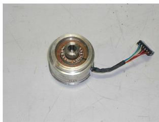
Figure 4: Siemens resolver.
